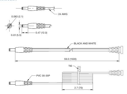
Wire type: VW-1 80°C 300 V L=1500 mm 2468, 22 AWG for 12 V ouput, 24 AWG for other outputs, 2C Black and White. Black - Negative, White - Positive
