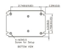
Each one of the 4 screw holes can be used as a PE connection for CLASS I application.
