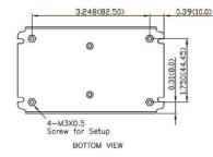
Each one of the 4 screw holes can be used as a PE connection for CLASS I application.
