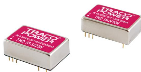
The THD-15N series models provide 15 Watt output power out of a very compact shielded metal case that occupies only 1 inch<sup>2</sup> of board space. The converters work with a high efficiency over the full load range and draw a very low input current at no load conditions. All models have a wide 2:1 input voltage range and a precisely regulated output voltage.
