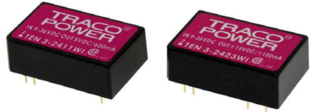
The TEN 3WI series is a family of dc-dc converter modules with 3W output power, featuring ultra wide 4:1 input voltage ranges of 9-36VDC or 18-75VDC. They come in a DIP-24 plastic package with industry-standard footprint. A high efficiency up to 84% allows operation ambient temperatures of  $-40^{\circ}\text{C}$  to  $+70^{\circ}\text{C}$  at full load.
