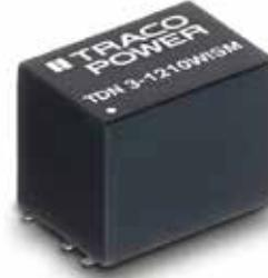
The TDN 3WISM Series comprises 3 Watt fully regulated, high performance DC/DC converters. They come in a compact cubical package of only 1.23 cm<sup>3</sup>. Full load operation is reliable up to 70°C environment temperature. With 1'600 VDC I/O-isolation voltage, external On/Off, and short current protection they cover a wide range of application when space is limited. The input of the converters is designed for a wide voltage range (4:1) and minimum load is not required.
