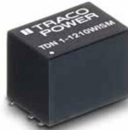
The TDN 1WISM Series comprises 1 Watt fully regulated, high performance DC/DC converters. They come in a compact cubical package of only 1.23 cm<sup>3</sup>. Full load operation is reliable up to 90°C environment temperature. With 1'600 VDC I/O-isolation voltage, external On/Off, and short current protection they cover a wide range of application when space is limited. The input of the converters is designed for a wide voltage range (4:1) and minimum load is not required.
