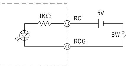
(B) Using external voltage source
