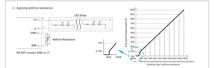
Note: 1. Min. duty cycle of output current is about 0.15%, and the dimming input is about  $6K\Omega$  or 0.6VDC, or 10V PWM signal with 6% duty cycle. 2. The duty cycle of output current could drop down to 0% when dimming input is less than  $6K\Omega$  or less than 0.6VDC, or 10V PWM signal with duty cycle less than 6%.
