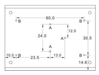
A=For fixture to din rail clip only B=For fixture to pcb/chassis only
