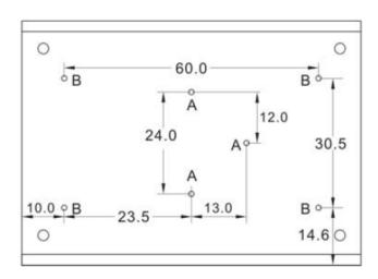
A=For fixture to din rail clip only
