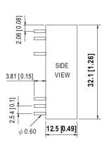
NOTE: Pin tolerance ±0.05mm
