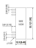
NOTE: Pin tolerance ±0.05mm
