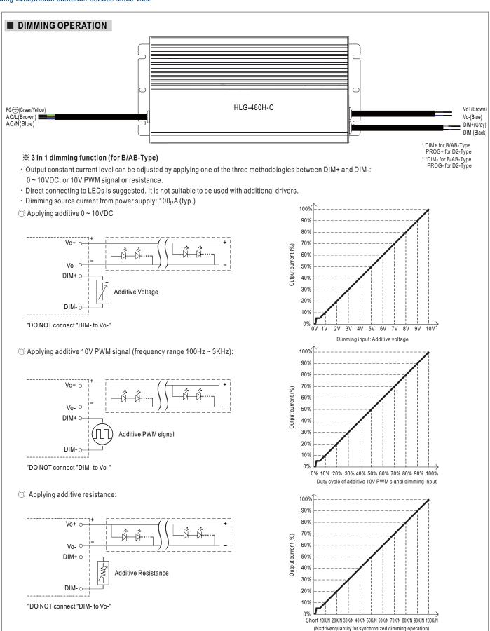
Note: 1. Min. dimming level is about 6% and the output current is not defined when 0% < Iout < 6%.
