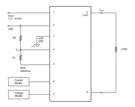
Operate with 5VDC Reference Voltage Variable output
