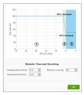
Area 1: Output is 100%, NTC > Start Point (temperature of LED module below Protection threshold)
