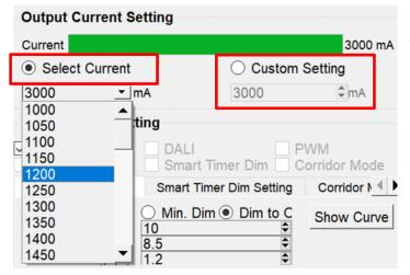
Output current can be changed either by selecting output current from the drop-down list or entering current value in the righthand column.
