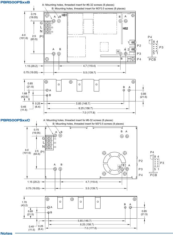
Input Connector - P1 Pin 1 G Pin 2 L Pin 3 Ν
