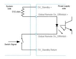
Figure 17. Global remote On\_Off connection
