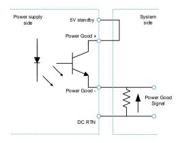
Figure 18. Power good signal sequence
