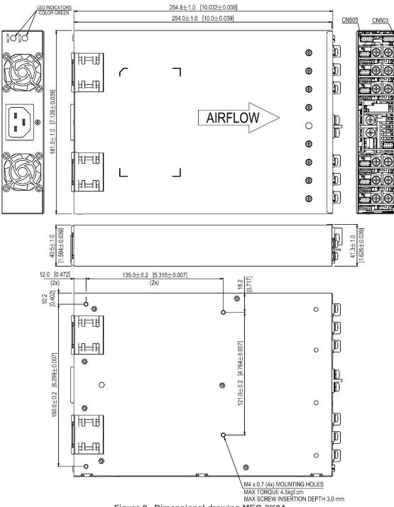
Figure 2. Dimensional drawing MEG-3K0A
