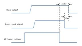
Figure 19. Power good signal connection
