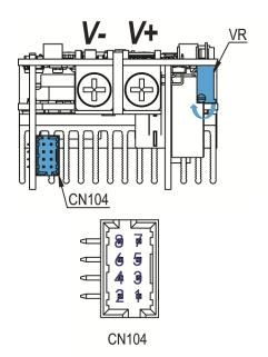
Figure 10. -x2 Module Connector
