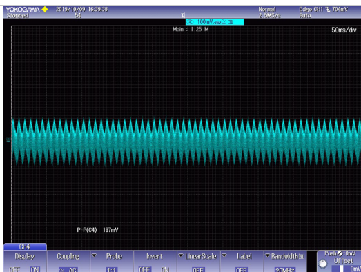
(a) 115V (measured value=187mV)
