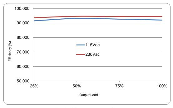
Fig. 1 Efficiency versus output load
