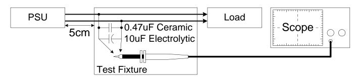
Fig. 3 Ripple & Noise measurement circuit
