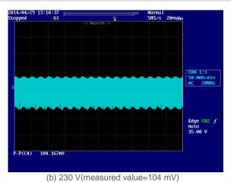
Fig. 2 Ripple & Noise example, 20 MHz BW
