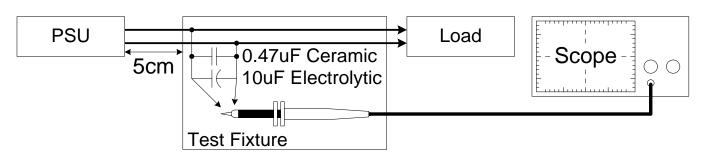
Fig. 3 Ripple & Noise measurement circuit
