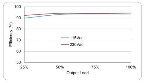
Fig. 1 Efficiency versus output load
