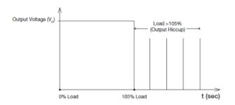
Additionally, if the Io is <250% but >110% for a prolong period of time (depending on the load), the Over Temperature Protection (OTP) will be activated due to high temperature on critical components. The power supply will then go into hiccup mode until the fault is removed; and, the input voltage is removed, then reapplied.
