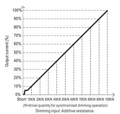
Note: 1. Min. dimming level is about 8% and the output current is not defined when 0% Lout < 8%.
