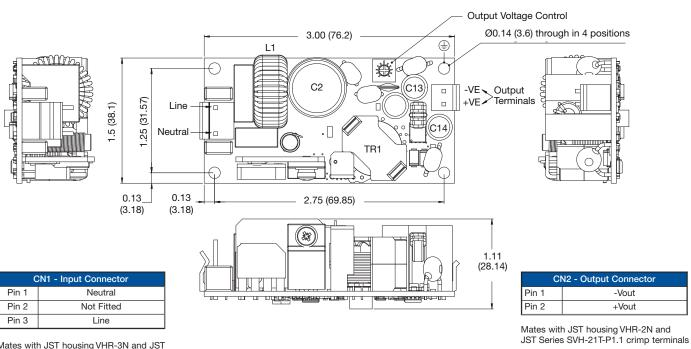
Mates with JST housing VHR-3N and JST Series SVH-21T-P1.1 crimp terminals
